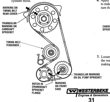
At this time, check that the moveable range of teeth on the oil pump sprocket is according to specifications.
