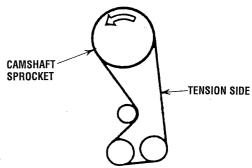
7. Loosen the temperorarily tightened tensioner nut on the water pump side 1 or 2 turns, and tension the belt making use of spring force.
