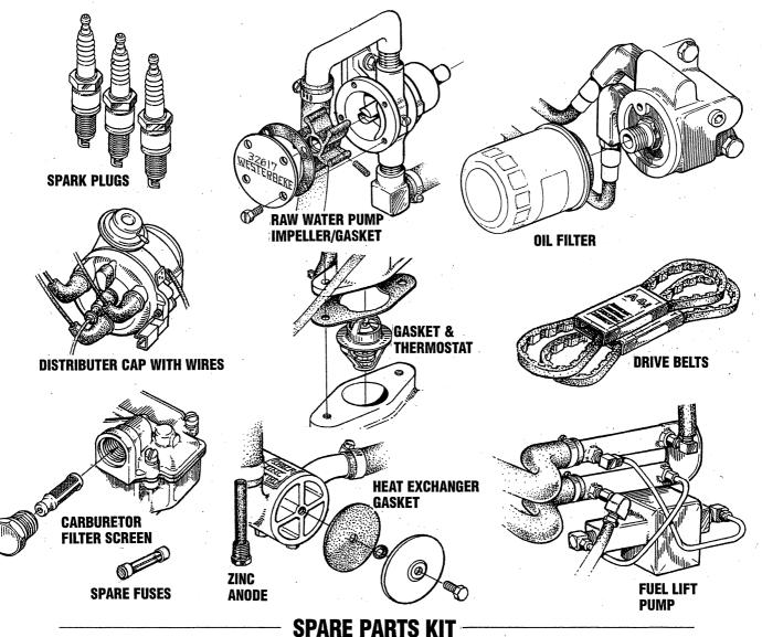
WESTERBEKE offers two Spare Parts Kits, each packaged in a rugged hinged toolbox. Kit A includes the basic spares. Kit B is for more extensive off-shore cruising.
