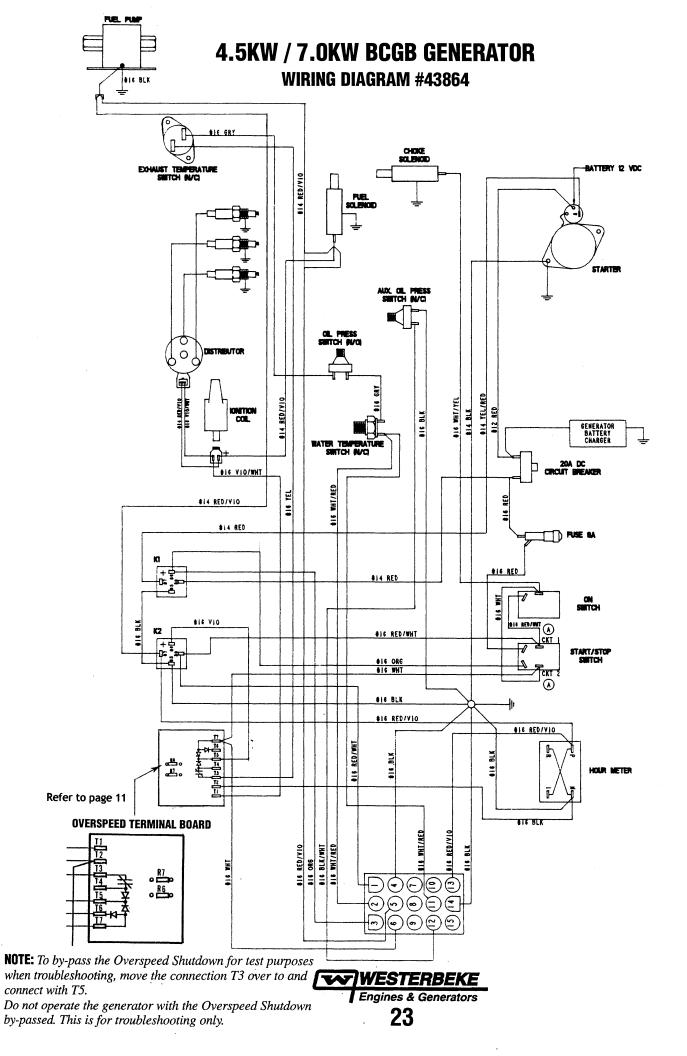
4.5KW / 7.0KW BCGB GENERATOR WIRING SCHEMATIC #43864
