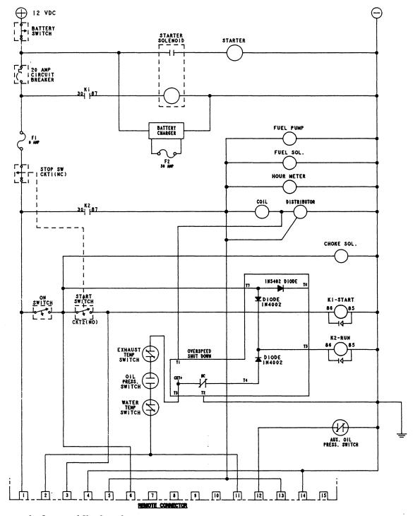
**NOTE:** To by-pass the Overspeed Shutdown for test purposes when troubleshooting, move the connection T3 over to and connect with T5.
