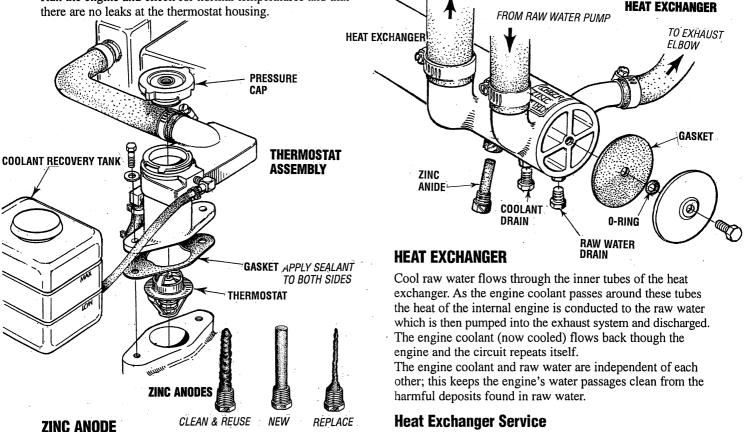
A zinc anode (or pencil) is located in the raw water cooling circuit within the heat exchanger. The purpose of the zinc anode is to sacrifice itself to electrolysis action taking place in the raw water cooling circuit, thereby reducing the effects of electrolysis on other components of the system. The condition of the zinc anode should be checked monthly and the anode cleaned or replaced, as required. Spare anodes should be carried onboard.
