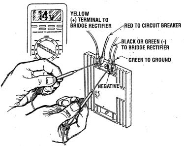
The generator supplies a continuous 17 amp charge from its battery charger to the starting battery. To test the battery charger put a multimeter between the positive (+) and negative (-) leads to the battery. It should indicate 13.5V to 14V with the engine running. If only the battery voltage is indicated, check that the battery charger terminal connections are tight. With the unit running, test between the (+) and (-) terminals for 13.5V to 14V. If no charge is indicated, replace the charger.
