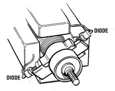
1. Rotating Field/Auxiliary Windings Single Capacitor 3.8 Ohm – Dual Excitor – 4.0 Ohm
