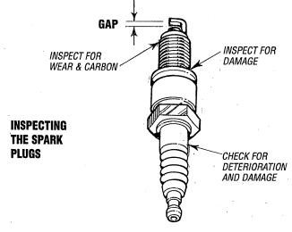
USE A 13/16" DEEP SOCKET WHEN REMOVING AND INSTALLING THE SPARK PLUG.
