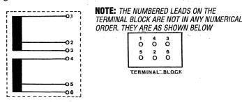
Group #1 - Measure resistance value between terminal with lead <math>#1 and terminal with lead #3. (Check that there is no continuity of Group #1 windings to the case ground.)
